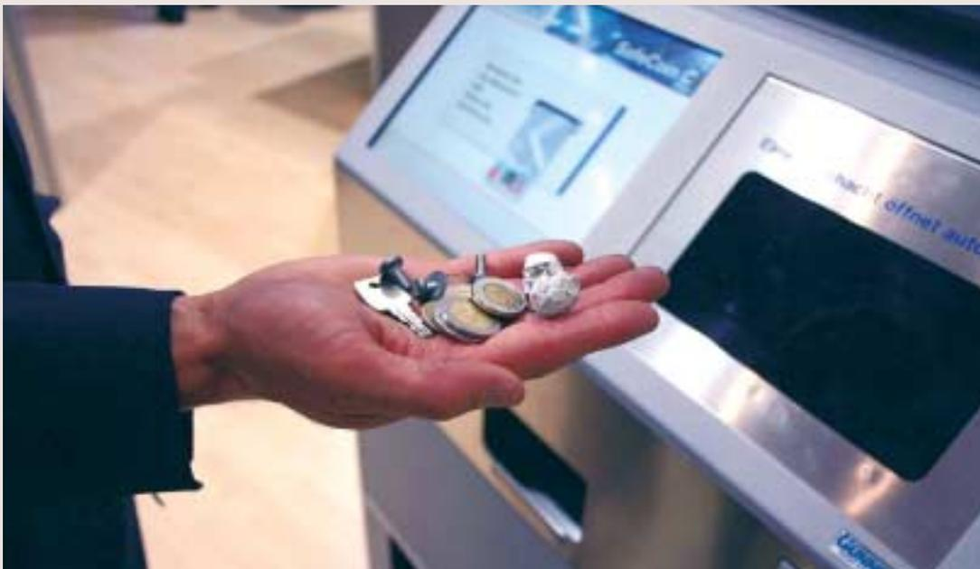
*One of the new products at Gunnebo's stand was the SafeCoin C, a coin deposit machine that can distinguish between different coin denominations and currencies thanks to highly reliable laser scanning. The machine also systematically filters out any foreign objects such as scraps of paper, screws or keys that are accidentally dropped into it.*
