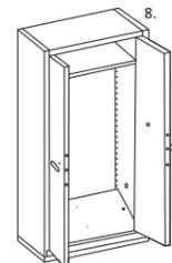
**STEP 8.** Insert the symmetrical inner base plate, covering the anchoring bolts and position shelves using shelf clips supplied in your kit.
