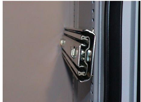
Pull out the slides on both sides and press the shelf onto the hooks on the slides.
