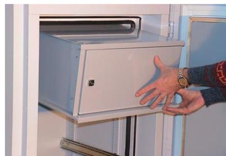
Fix the compartment to the cabinet with the enclosed four screws. Don't tighten the screws to hard; it may deform the wall of the compartment. Adjust the screws to get an even slit around the door which guarantees a smooth operating compartment door and lock.
