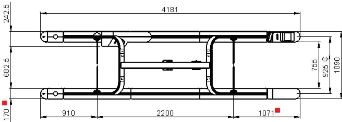
Please note: this is an example of one possible implementation. Some dimensions can vary according to requirements. Dimensions which cannot be altered have been marked with ■
